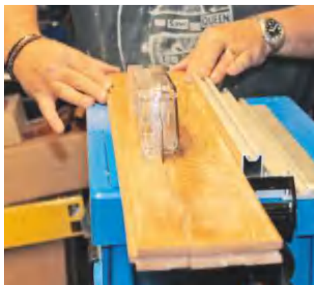
▲ Ripping solid oak flooring is well within the saw's remit
